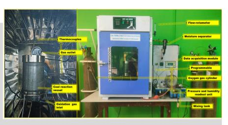
The method involves studying the thermal evolution of coal undergoing spontaneous combustion under ambient environmental conditions of humidity, moisture, particle size, gas concentration, and gas velocity. This patent is the outcome of the R&D project undertaken jointly by BIT Sindri and IIT (ISM) Dhanbad with the funding support of TexMin, IIT (ISM) Dhanbad.
